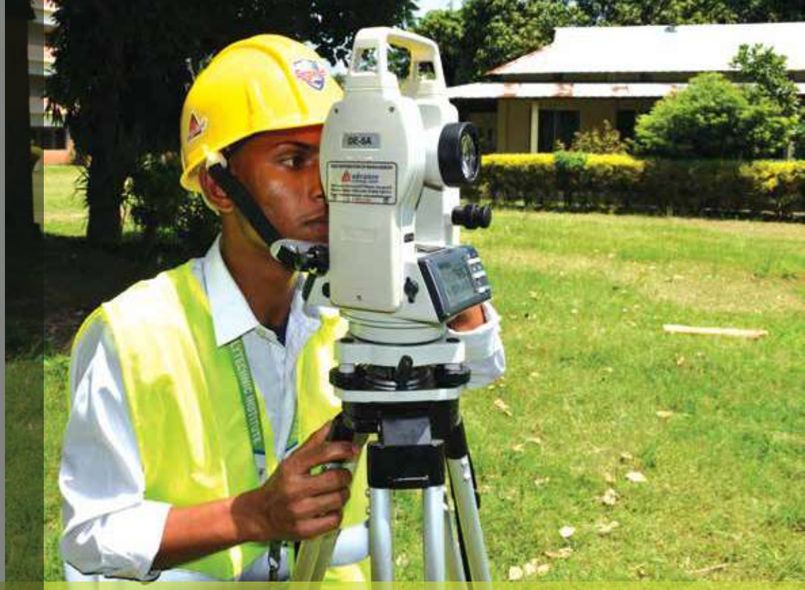
A student, belonging to Civil Technology, practices theodolite machine to estimate the height of a building.
